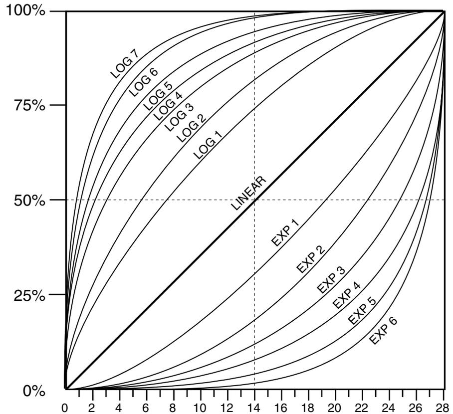
The speed curves can be used in 14, 28 and 128 speed step modes.
